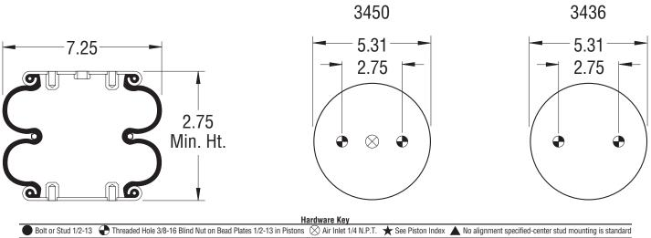
🛞 Combination Stud/Air Inlet Stud Outside Thread is 3/4-16 🛛 Studs Inside Thread (Air Inlet) is 1/4 N.P.T. Exceptions will be noted on Part View as 🛞
